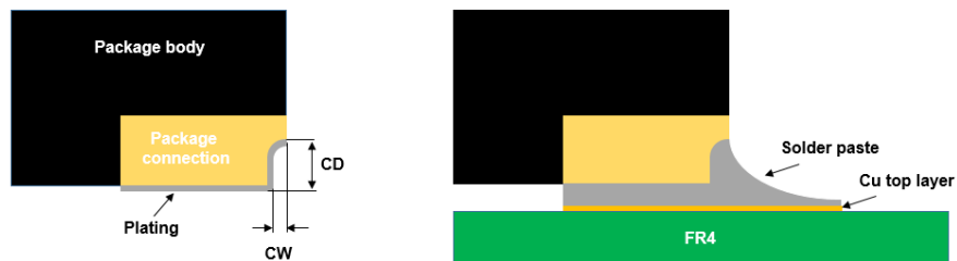
Figure 17. Wettable flank profile
