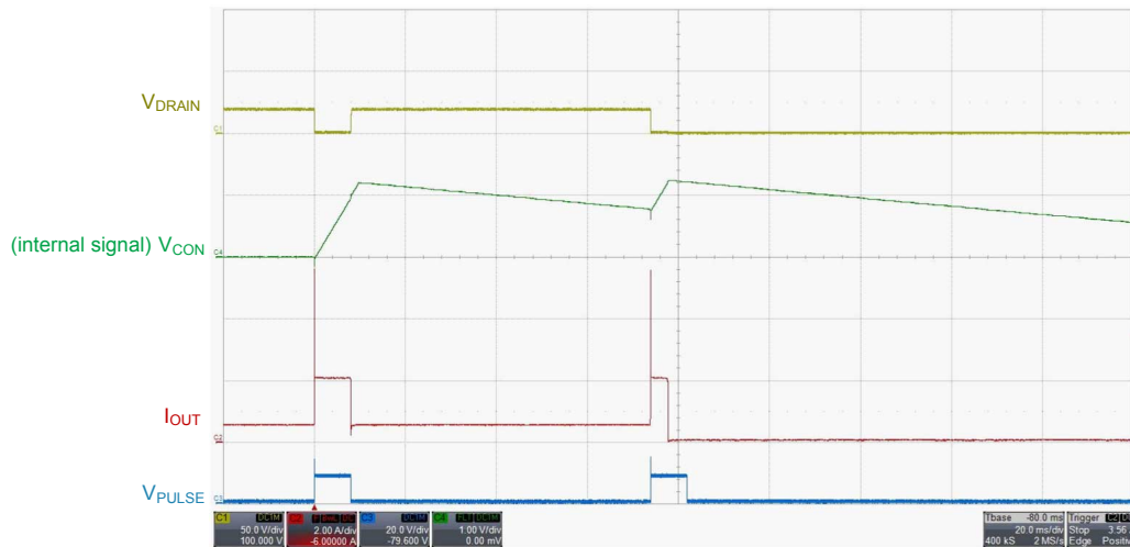
Figure 8. Behavior under repetitive overloads (magnification)
