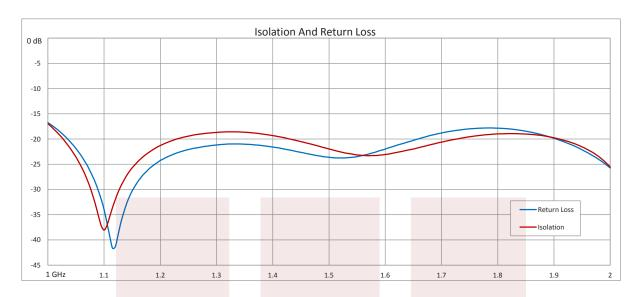
High Power Circulator SMA Female With 18 dB Isolation From 1 GHz to 2 GHz Rated to 50 Watts from Fairview Microwave is in-stock and available to ship same-day. All of our RF/microwave products are available off-the-shelf from our ISO 9001:2008 certified facilities in Lewisville, Texas. Fairview Microwave is RF on-demand.
