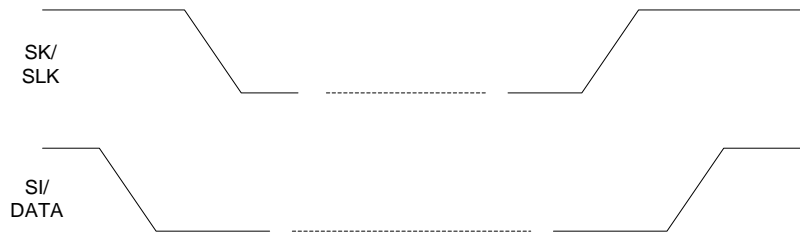
Figure 24: Timing of 2-WIRE START and STOP Condition
