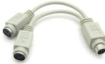
Figure 4-26 Y-Cable use for both Keyboard and Mouse
