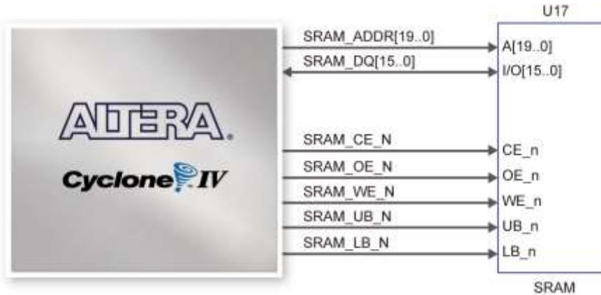
Figure 4-33 Connections between FPGA and SRAM
