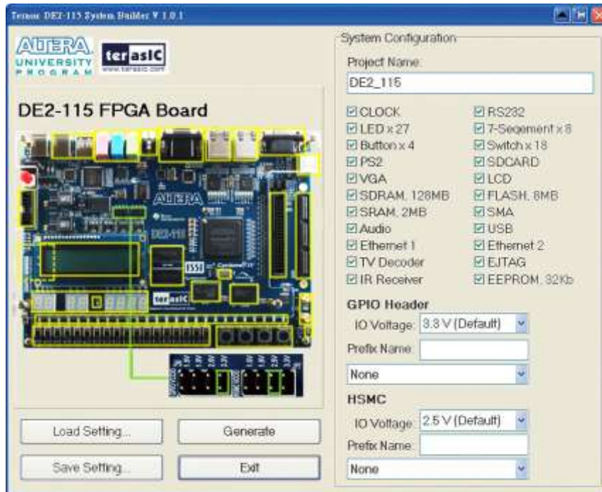
Figure 5-2 The DE2-115 System Builder window
