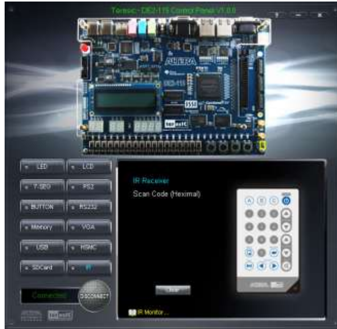
Figure 3-14 Testing the IR receiver using remote controller
