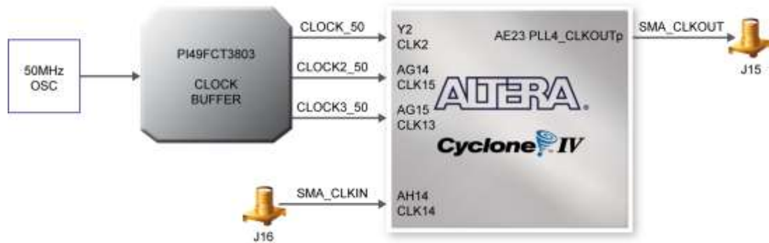
Figure 4-11 Block diagram of the clock distribution
